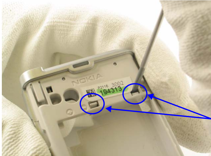
IHF assembly retention snaps
