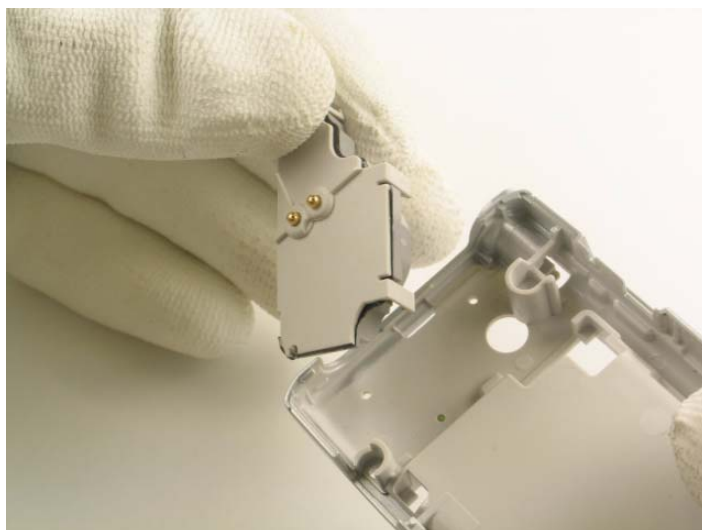
Lift IHF assembly from the D-cover
